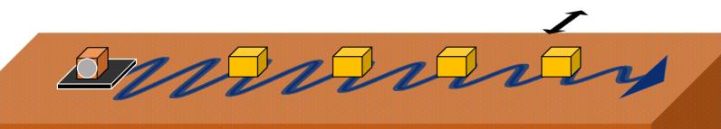
40Hz, Body wave in shear direction
