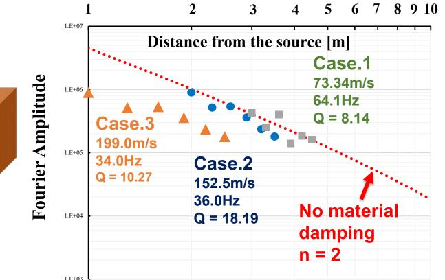
$\succ$  Calculate the energy decay constant  $\alpha_0$  by comparing the Fourier amplitude near the peak frequency with the propagating distance, then wavenumber conversion **k** The range of shear wave velocity was 73.3~199 m/s  $\succ$  The calculated energy attenuation constant  $\alpha_0$  was 1.39  $\times$  $10^{-3} \sim 10.1 \times 10^{-3}$ , about 20~50% of the amplitude was damped for every wavelength advanced
