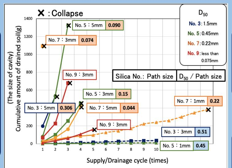
✓ The ratio of particle size to path size is related to the degree of soil drainage.
