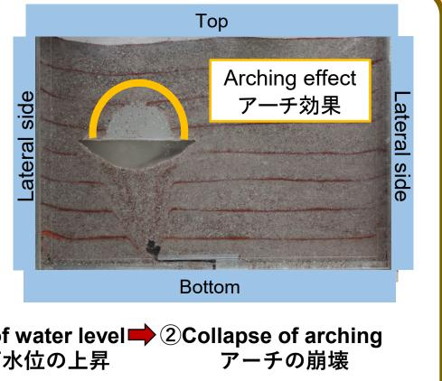
**1**Rise of water level → **2**Collapse of arching 地下水位の上昇
