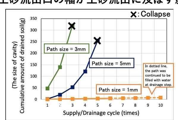
The degree of Soil drainage 土砂流出の程度 Path size 3 mm > 5 mm > 1 mm土砂流出口の幅
