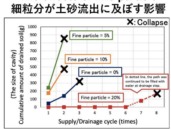
In the case in which fine particle rate is 20%, the tendency of soil drainage was smaller.
