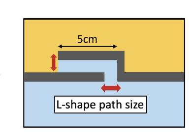
Reproduction of water leakage gap in a buried pipe
