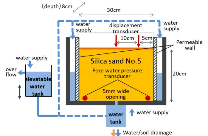
1. Model ground was made in the soil chamber using uniform sand.
