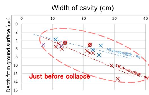
Wet uniform sand above a cavity collapses due to its self weight, when the ratio of average depth and cavity width becomes below 0.2 to 0.3.
