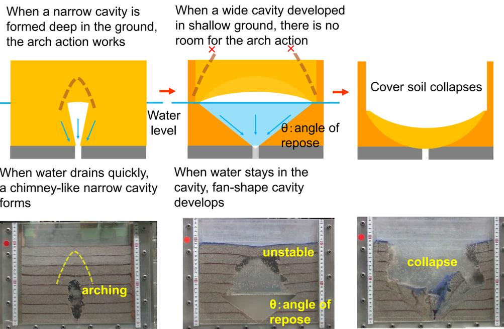
Change of water level, or high water level are one of main factors for cavity expansion
