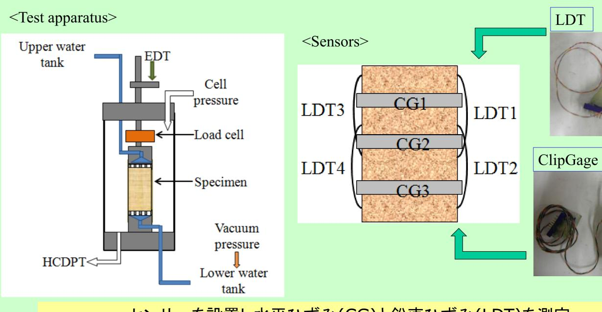
センサーを設置し水平ひずみ(CG)と鉛直ひずみ(LDT)を測定 微小ひずみ繰り返しにより実験中のヤング率とポアソン比を算出 ClipGages are for horizontal strain and LDTs are for vertical strain Young's Modulus and Poisson's Ratio were estimated from these sensors by applying the cyclic loadings.
