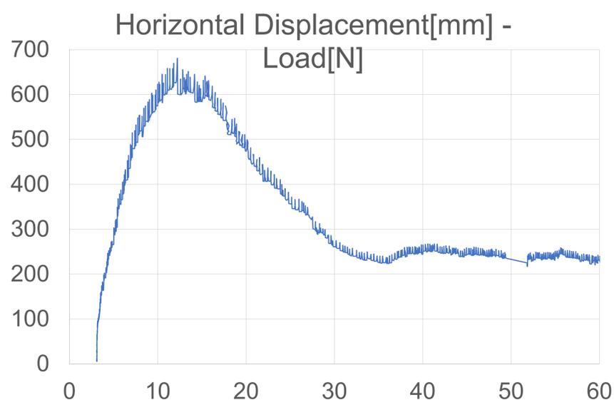
This result is the sample in case of **111Pa(10N) loading pressure**, for the volcanic soil include gravel and using handy oil jack, **large(30cm) shear box**. The jack can be moved only little bit by one paddling. And the many small pulse that you can see in the left graph means the timing that the jack started moving. As you can see, we can easily get the **residual strength** (around 250N) and the **peak strength** (around 630N) from the graph.
