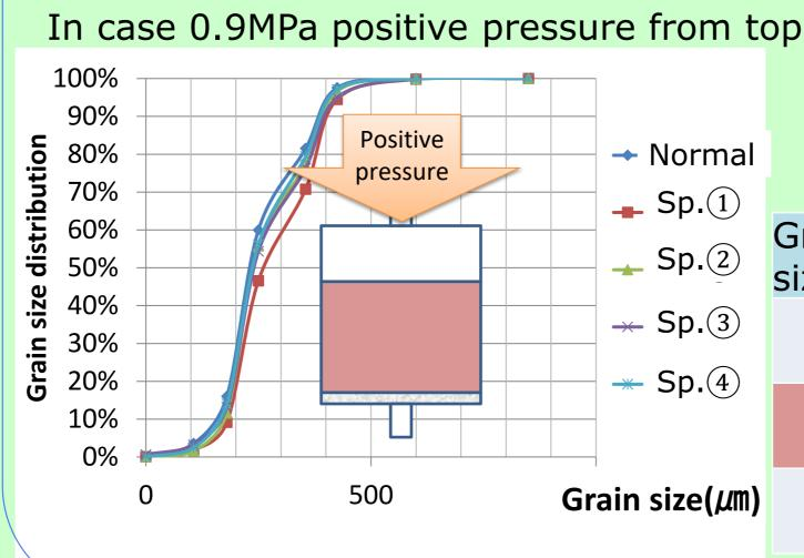
Test time: 3 minutes Average flow rate: 45.2cm<sup>3</sup>/s Water flow direction
