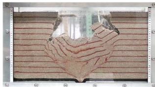
Simulation of road cave-in accident by laboratory model test
