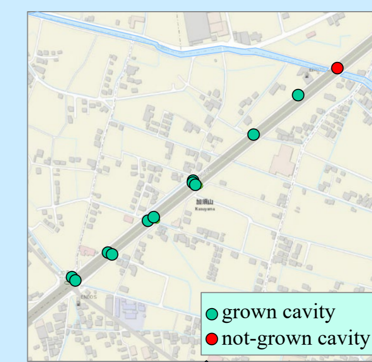
水路に交差する地点に発生した空洞 A cavity growth which occurred at the intersection of a road and a channel.
