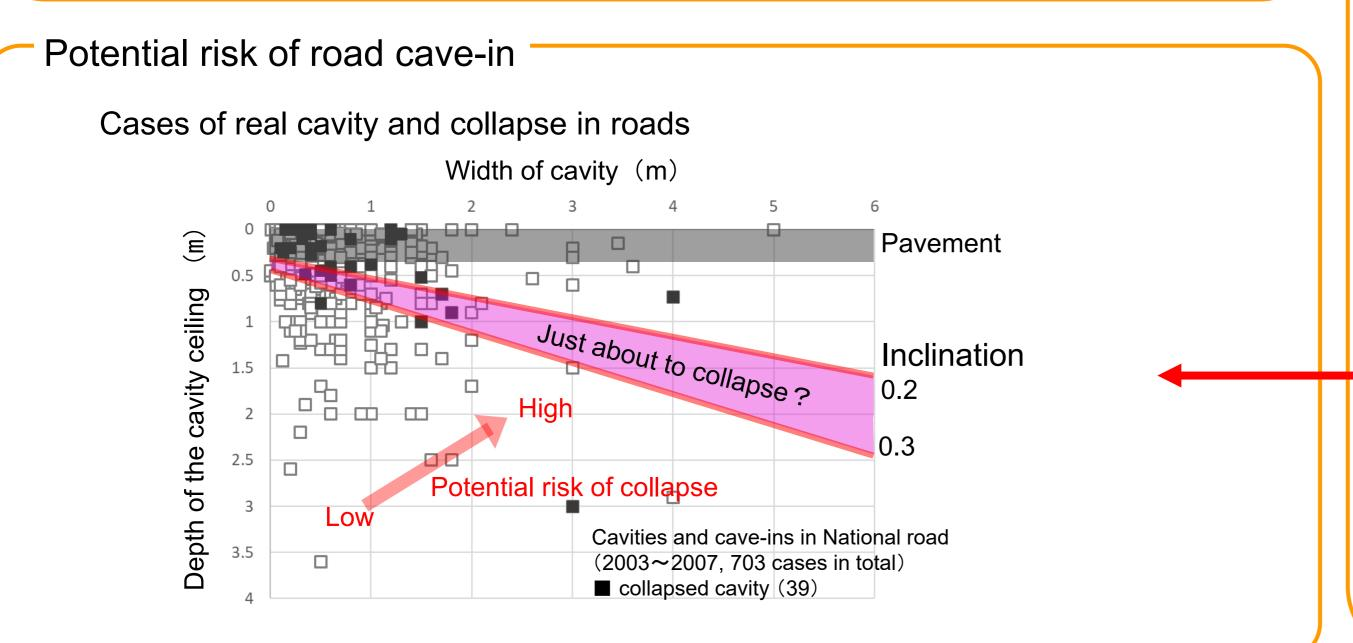
When the thickness of covering soil is large enough compared to the width of cavity, a cavity is stable as the ground arching and apparent cohesion seems to work.
