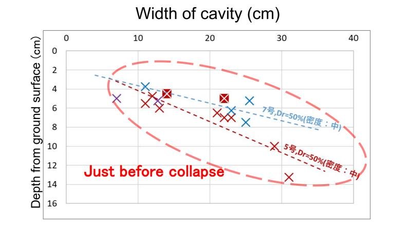
Wet uniform sand above a cavity collapses due to its self weight, when the ratio of average depth and cavity width becomes below 0.2 to 0.3.
