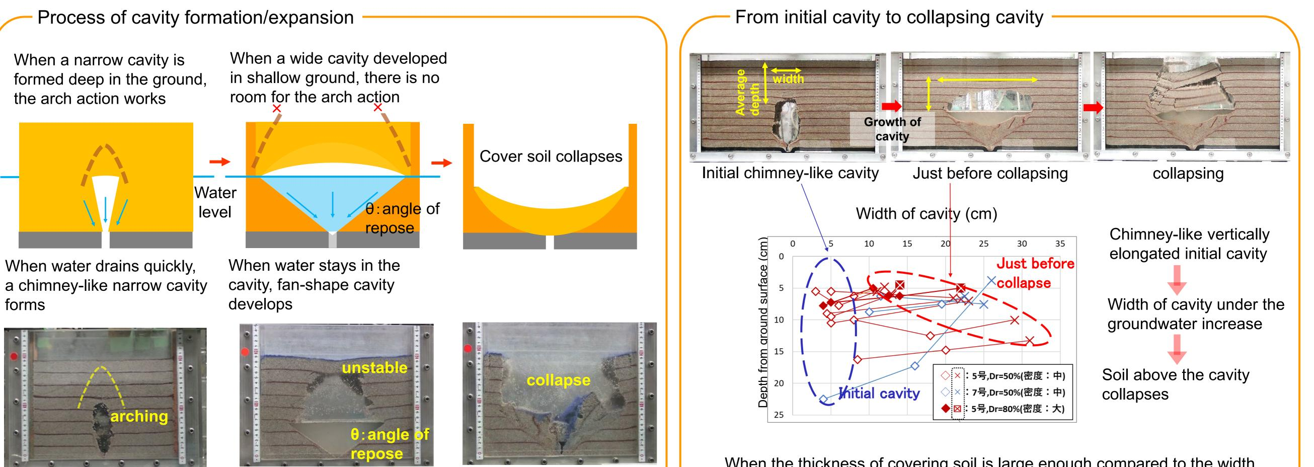
Change of water level, or high water level are one of main factors for cavity expansion
