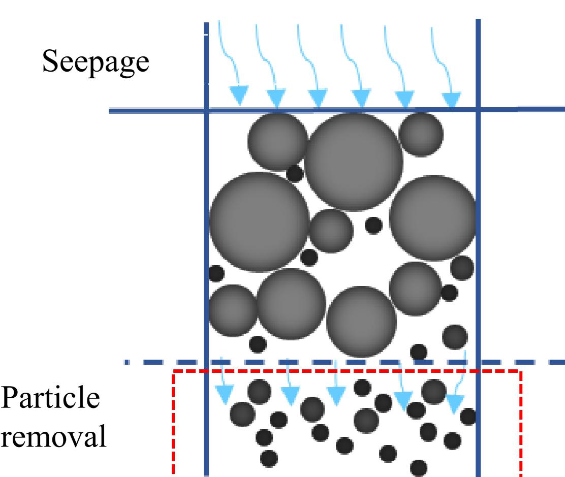
Detachments of soil particles from the **main structure** inside the ground due to mechanical or chemical actions of **seepage flow**
