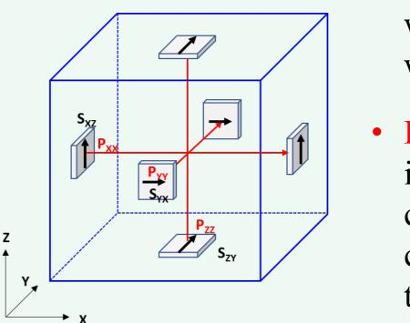
• The present test setup provides three types of Pwaves, i.e.  $P_{XX}$ ,  $P_{YY}$  and  $P_{ZZ}$ , and three types of Swaves, i.e.  $S_{YX}$ ,  $S_{XZ}$  and  $S_{ZY}$
