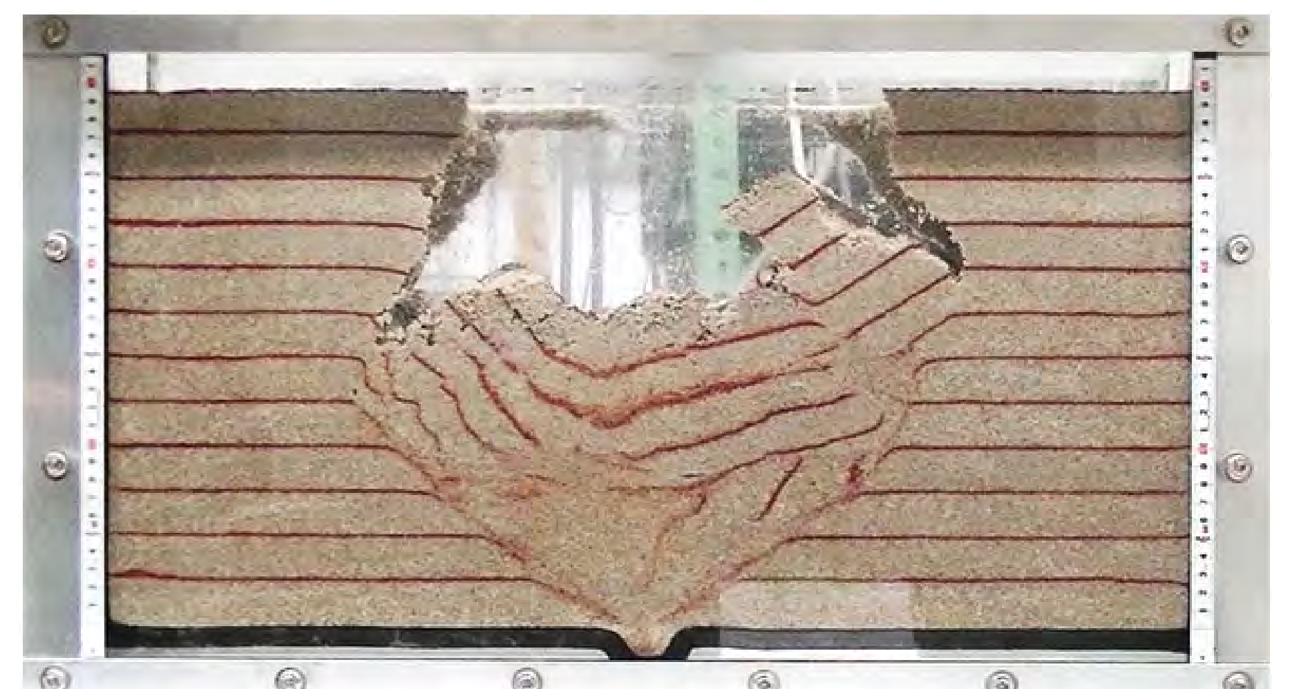
Simulation of road cave-in accident by laboratory model test
