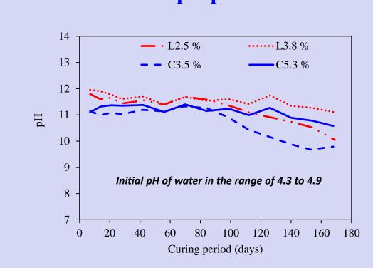
pH values of soaking acid water had increased up to 12 in lime treated soils and 11 in cement treated soils initially, while those values started to decrease gradually with the curing period.
