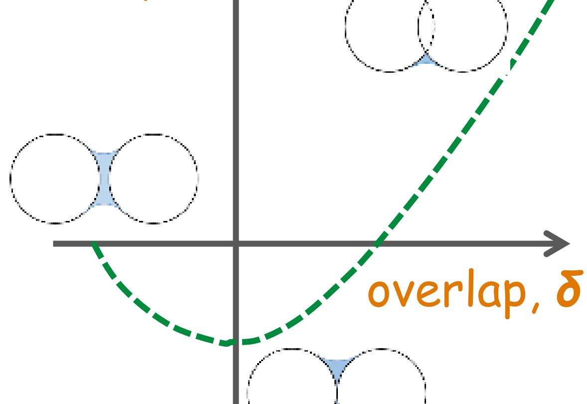
$$F = \text{capillary force} + \text{Hertzian contact force}$$
