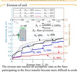
Rate of erosion is density dependent.
