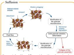
Seepage induced loss of fine particles with no change in volume and an increase of hydraulic conductivity
