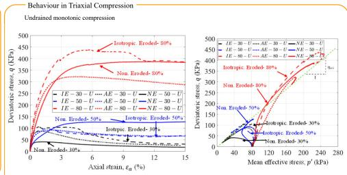
In the undrained triaxial compression tests it was observed that eroded soil shows higher peak strength due to cushioning effect at small strain and becomes more collapsible than uneroded soil at higher strains due to removal of fines and particle rearrangement during the erosion.
