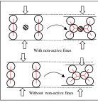
Elastic yield surface seemed to be expanded for eroded soil specimen. It could be due to action of suffusion and fine removal.
