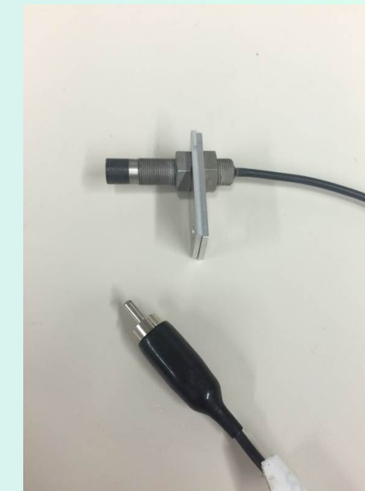
Gap Sensor (Shear modulus measurement during small torsional cyclic loadings)
