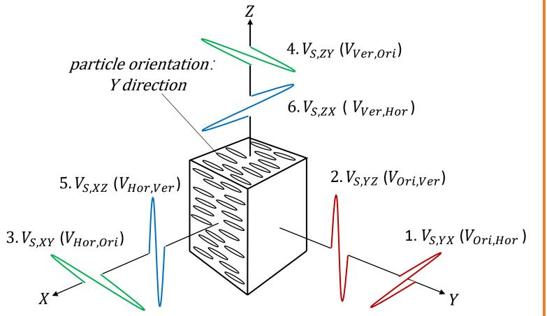
The first and second subscripts indicate the direction of the S-wave propagation and oscillation, respectively, i.e., v<sub>Ori,Hor</sub> represents the shear waves that propagate along particle orientation and oscillate within the horizontal plane;  $v_{Hor,Ver}$  means the shear waves that propagate perpendicularly to the particle orientation within the horizontal plane and oscillate along the vertical direction.
