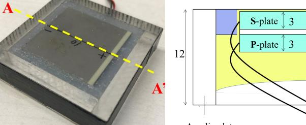
Shear Plate Transducer
