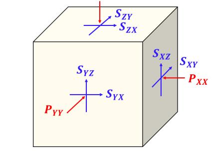
Considering both P- and S-waves, there are nine types of • elastic wave components as illustrated the left hand.
